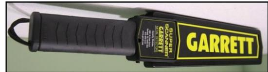
Figure2: The handheld metal detector should be used if the ferromagnetic detector is not functioning.
